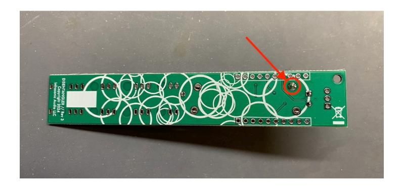
Once you've verified the slider is flat and flush, finish soldering the rest of the joints for the slider pins (7 in total).
