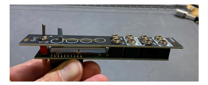
Once the panel is attached to the jacks and switch with the nuts, make sure once more that everything is aligned, parallel, and flush to both the panel and PCB, then flip the assembly over carefully and solder all the joints on the jacks and the switch. If anything is not aligned when you begin soldering, it can be tricky to fix, so it's very important to triple-check.
